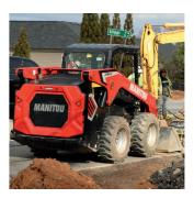
**Counterweight** A rear bumper counterweight improves productivity and protects the rear of the machine from accidental damage. Optional side counterweights can further increase operational capacity.
