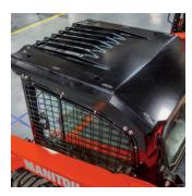
FOPS Level 2 For the users that need level 2 FOPS an optional level 2 heavy duty bracket delivers the protection they need. Bracket also protect the front LED work lights.
