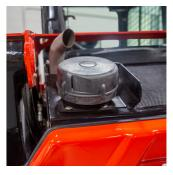
**Pre-cleaner** Reduce engine wear and TCO in dusty environments by adding an engine pre-cleaner.
