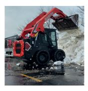
**Bucket self-leveling** Automatically maintain the bucket position when raising the lift arms.
